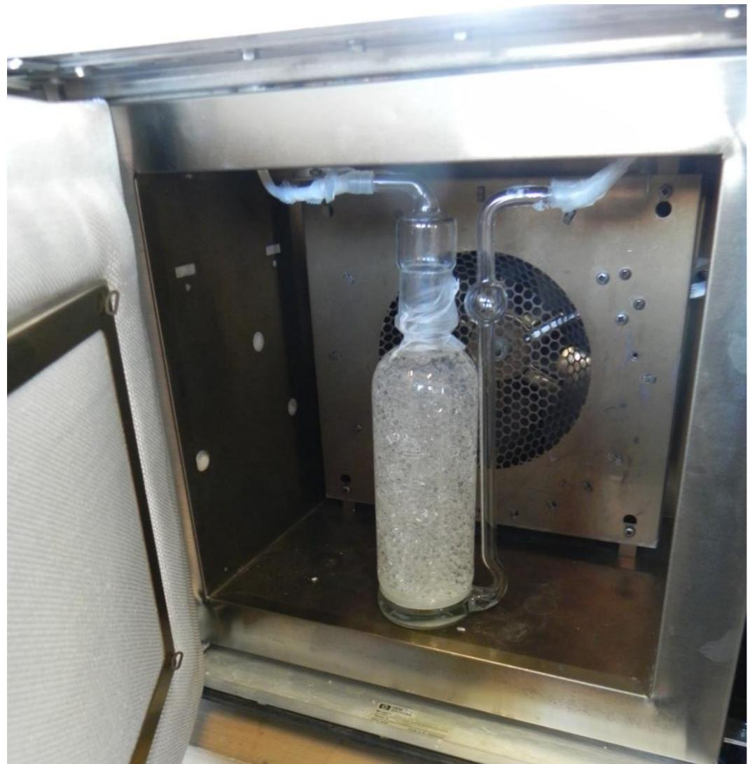
Wet process : absorption on solvent
