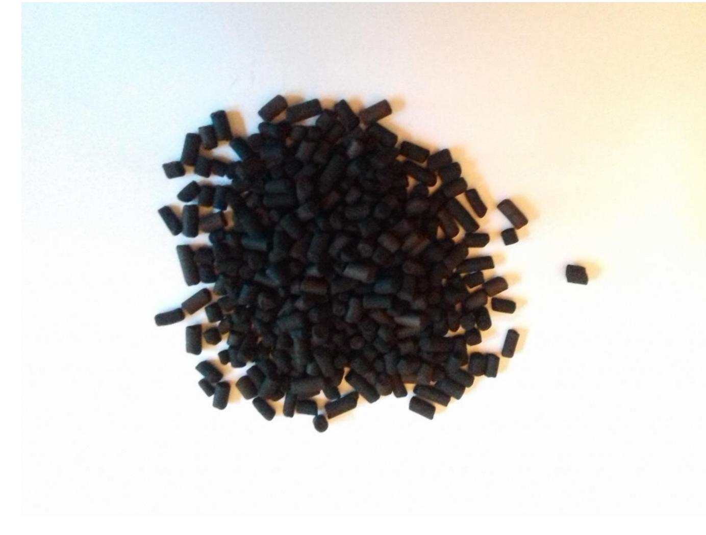
Dry process : adsorption on activated carbon.
