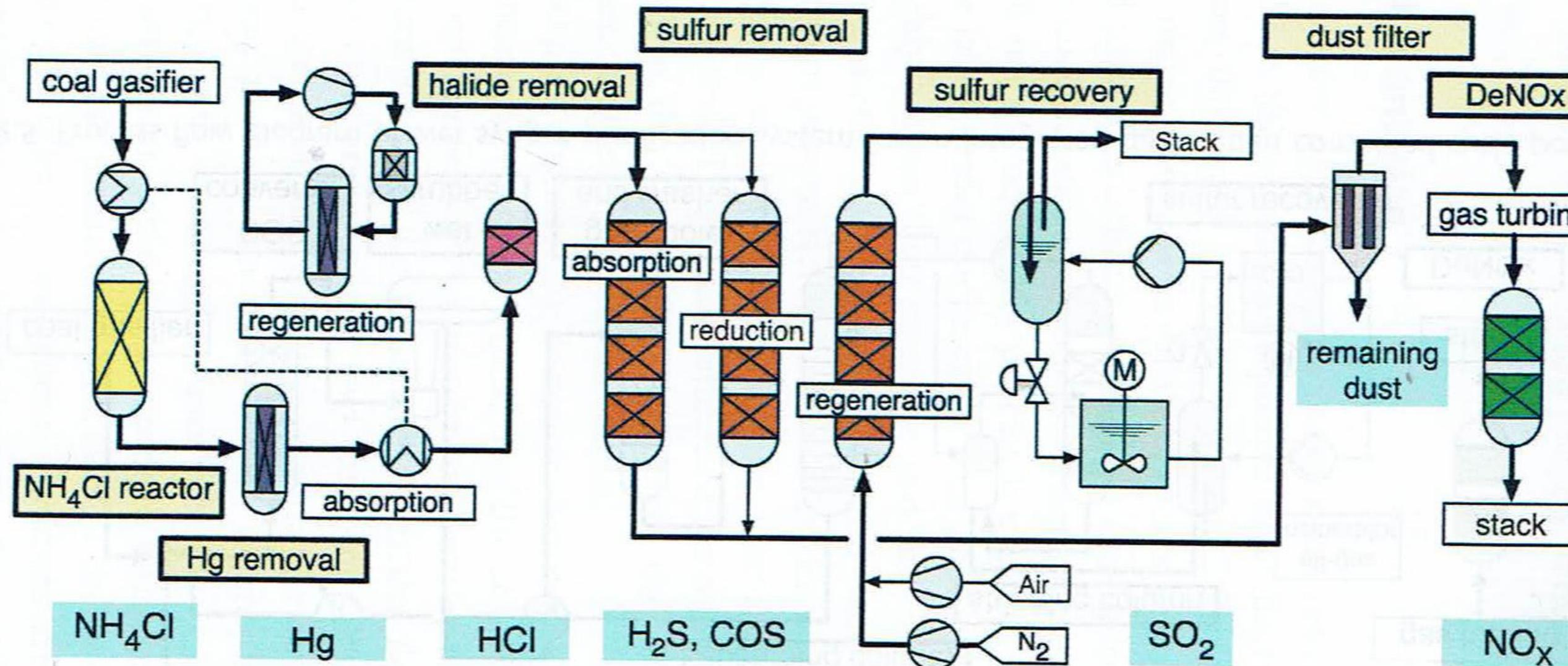
Figure 2.6 Process flow diagram of dry syngas purification system for an integrated gasification combined cycle power plant.
