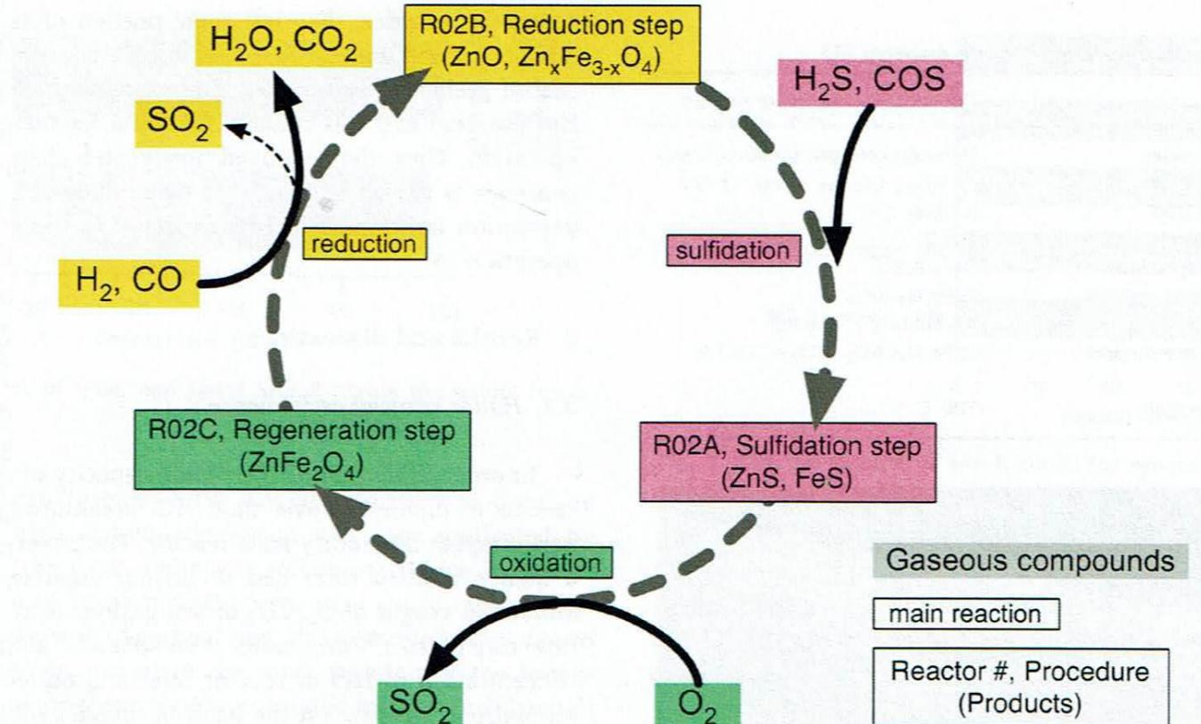
Fig. 3. Schematic diagram of the cyclic operation of the sulfur removal unit.
