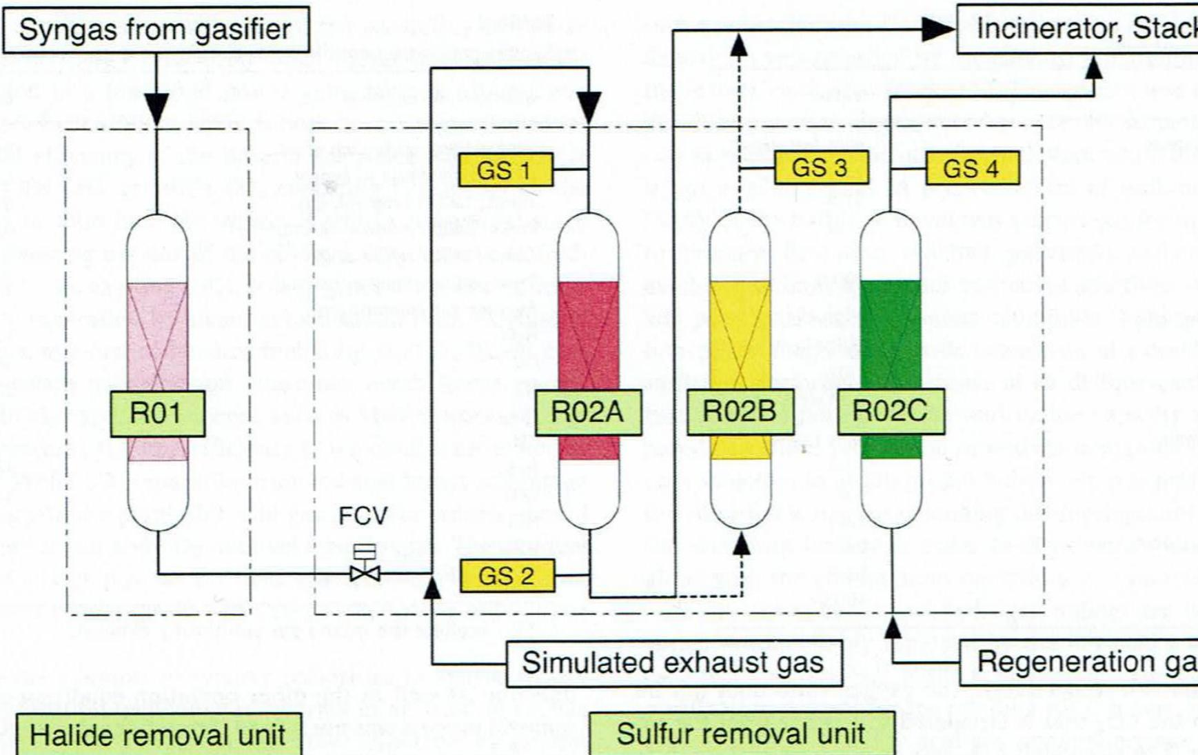
Fig. 2. Dry acid gas removal test facility installed at the  $\text{O}_2/\text{CO}_2$ -blown gasifier test plant.
