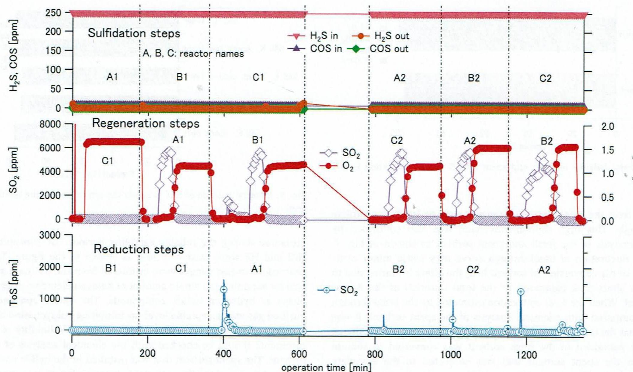
Fig. 10. Comprehensive performance test results obtained for the sulfur removal unit during 1st and 2nd cyclic operation of three reactors at the syngas test.
