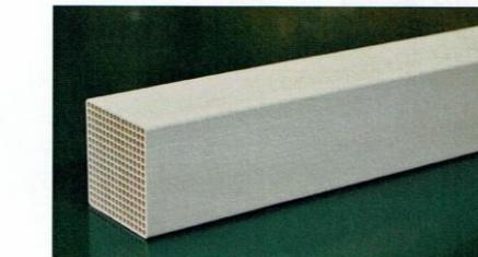
Fig. 5. Honeycomb desulfurization sorbent subjected to the syngas test.
