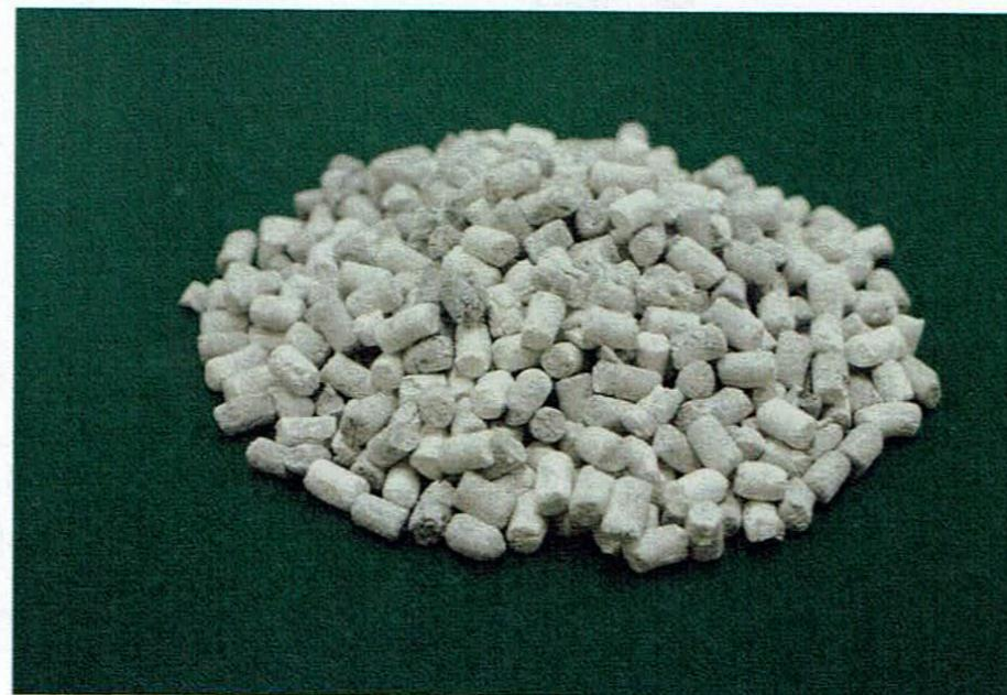
Fig. 4. Halide removal sorbent (SAS K) subjected to the syngas test.
