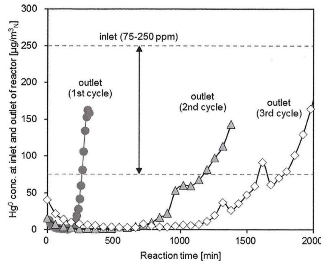
Fig. 5. Mercury breakthrough curves of the pre-sulfidized A-CBS honeycomb in three cyclic tests.
