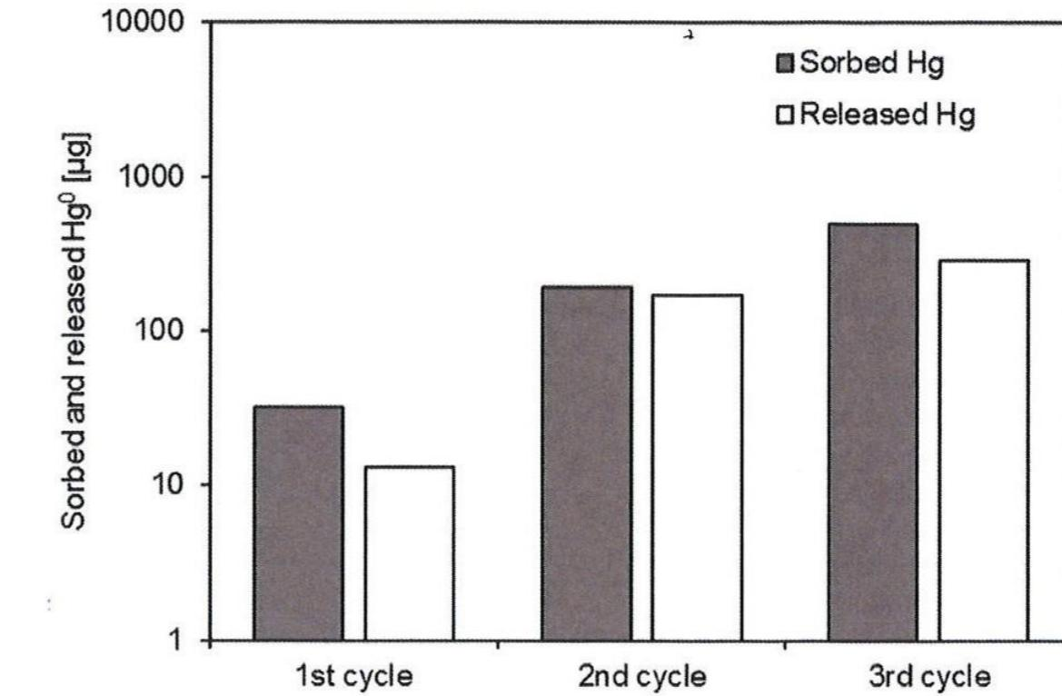
Fig. 7. Mercury balance obtained by gas analysis during the sequential operation using an A-CBS honeycomb.
